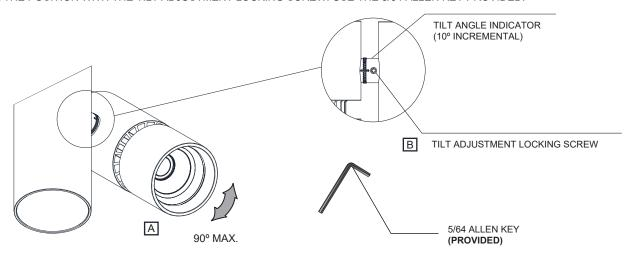
NOT UNLOCKING THE LOCKING SET SCREW TO CHANGE THE TILT ANGLE WILL CAUSE INTERNAL DAMAGE TO THE PROJECTOR.
