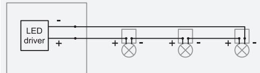
Luminaires must be connected on separate channels (1-4). Multiple luminaires can be connected in series on a channel (home run or fixture chain). Do not exceed the wattage and voltage range on each channel.
