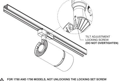
TO CHANGE THE TILT ANGLE WILL CAUSE INTERNAL DAMAGE TO THE PROJECTOR.
