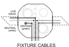
**!** If the wires for 0-10V dimming are not used, protect wire ends with twist connectors.
