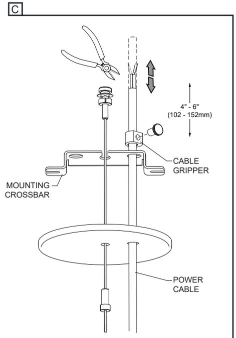
D- PASS THUMB SCREW INTO THE MOUNTING CROSSBAR KEY HOLE WITH LOCK WASHER ON TOP. HOLD SUSPENSION CABLE DOWN IN POSITION AND SECURE WITH THE PROVIDED NUT.
