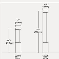
Stick is a family of cylindrical bollards with a simple and essential design, characterised by perfect uniformity of light all round. Available in three different sizes, each in two versions, single and double emission, Stick is particularly suitable for residential areas and guarantees a diffuse and homogeneous light beam. The Stick family, for its aesthetic and dimensional characteristics, completes the Microlighting collection designed to enhance outdoor residential spaces.
