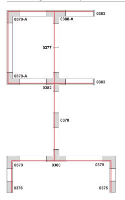
The track is polarized and is manufactured with identifying ridge (red line on this example). Different connector models must be ordered to make sure the polarization is respected throughout the complete track configuration.
