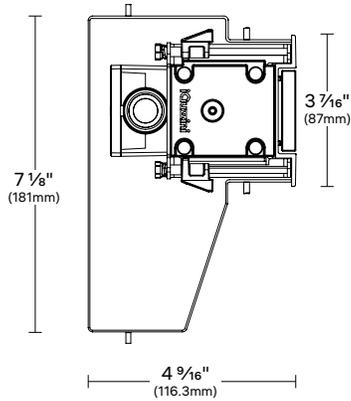
**M3 - Back box installation with safety cable installation**
