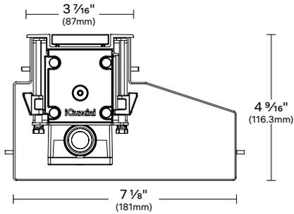
**M2 - Back box installation with safety cable installation**
