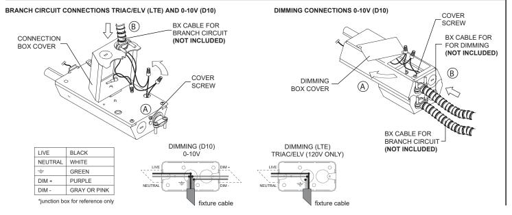
C- CLOSE THE CONNECTION BOX COVER OR DIMMING BOX COVER AND FASTEN WITH THE COVER SCREW. D-PASS THE CABLE LOOP THROUGH THE ATTACHEMENT CLIP OF THE CONNECTION BOX.
