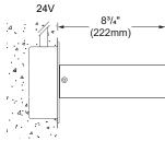
JB-REM - 4" junction box with remote power supply. Mounting adapter plate for junction box installation. Min 11/2" (38mm) deep.
