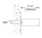
DF-REM - Direct feed with remote power supply. Connections made inside fixture (18AWG only). Ø3/8" power cable. Installed directly to surface.
