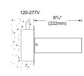
JB-UNV - 4" junction box with integral power supply. Mounting adapter plate for junction box installation. Min 11/2" (38mm) deep
