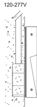
**JB-UNV** - 4" junction box with integral power supply. Mounting adapter plate for junction box installation. Min 1½" (38mm) deep
