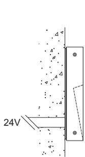
**DF-REM** - Direct feed with remote power supply. Connections made inside fixture (14-18AWG only). Max Ø3/8" power cable. Installed directly to surface.
