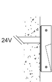
**DF-REM** - Direct feed with remote power supply. Connections made inside fixture. Max 2x18AWG. Installed directly to surface.
