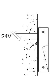
**FW-REM** - Fixture whip to remote power supply. Installed directly to surface with recessed pipe, or electrical conduit.
