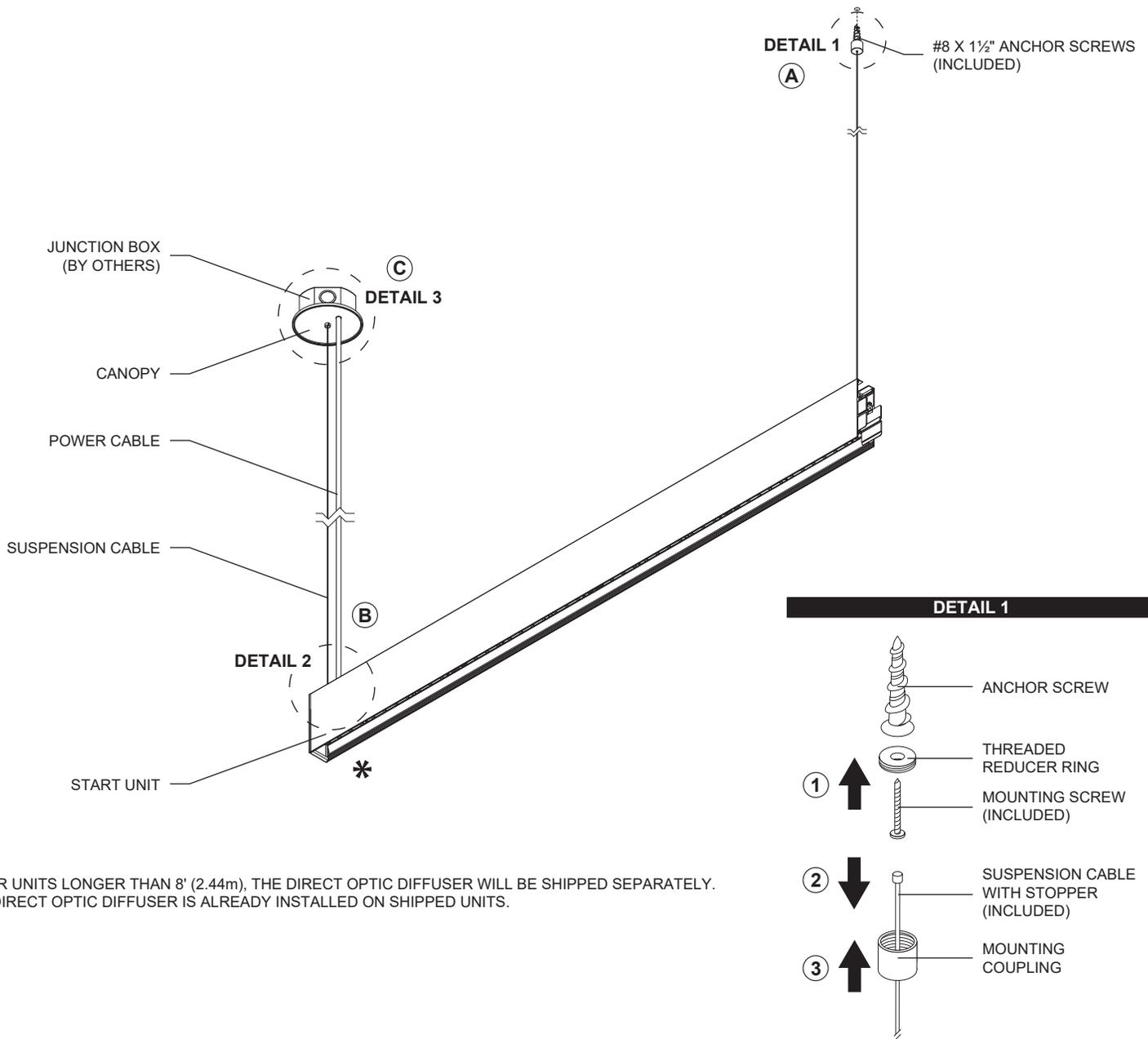
\*FOR UNITS LONGER THAN 8' (2.44m), THE DIRECT OPTIC DIFFUSER WILL BE SHIPPED SEPARATELY. INDIRECT OPTIC DIFFUSER IS ALREADY INSTALLED ON SHIPPED UNITS.
