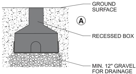
A - INSTALL RECESSED BOX OPENING FLUSH WITH SURFACE. **ALLOW 12" OF GRAVEL BELOW FOR DRAINAGE.**
