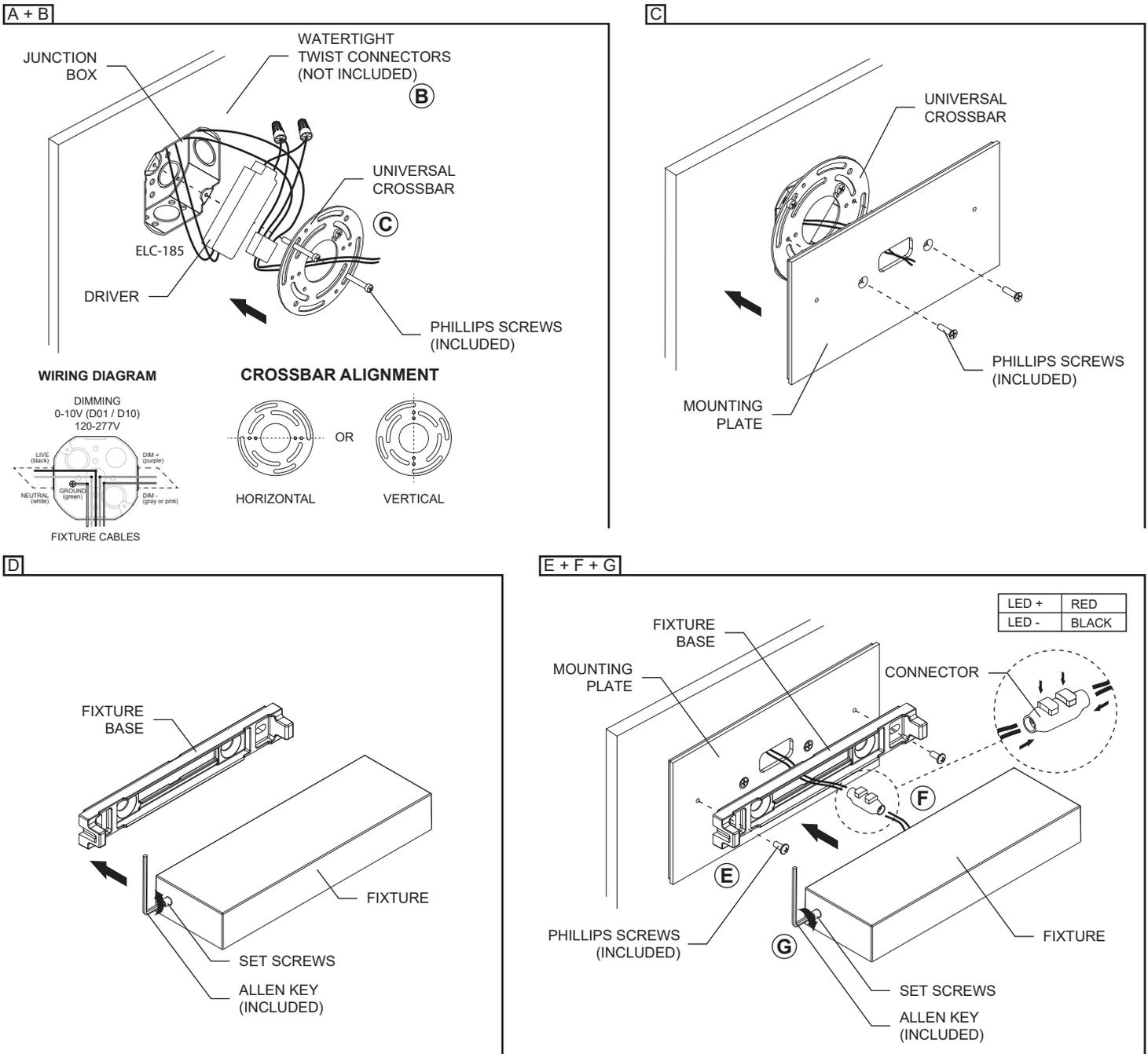
**⚠ DISCONNECT THE MAIN LINE BEFORE WIRING SECONDARY CONNECTORS.**
